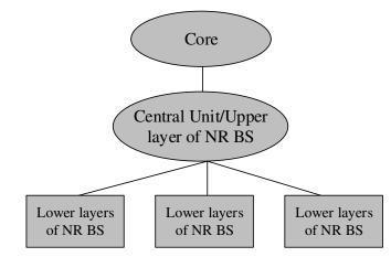
It was identified in [1] that The functional split between the Central Unit and lower layers of NR BS nodes may depend on the transport layer.
