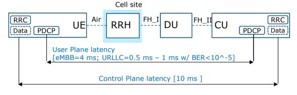
**5G User plane latency [38913]** - The time it takes to successfully deliver an application layer packet/message from the radio protocol layer 2/3 SDU ingress point to the radio protocol layer 2/3 SDU egress point via the radio interface in both uplink and downlink directions, where neither device nor Base Station reception is restricted by DRX (Discontinuous Reception occurring when in Idle mode for accomplishing with "paging" process).
