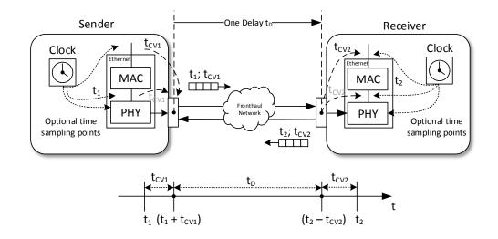
• The sender of the service message will sample the local time (t1) and include a compensation value (tcv1) and send it to the receiver.
