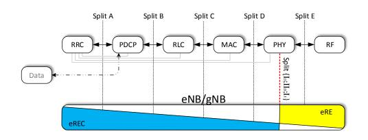
The major difference between Split  $I_{\rm D}$  and  $II_{\rm D}$  is that the data in Split  $I_{\rm D}$  is bit oriented and the data in split  $II_{\rm D}$  and  $I_{\rm U}$  is IQ oriented.
