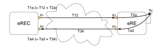
T12 is the transport network delay of a user data packet between eREC (R1) and eRE (R2) in DL direction.
