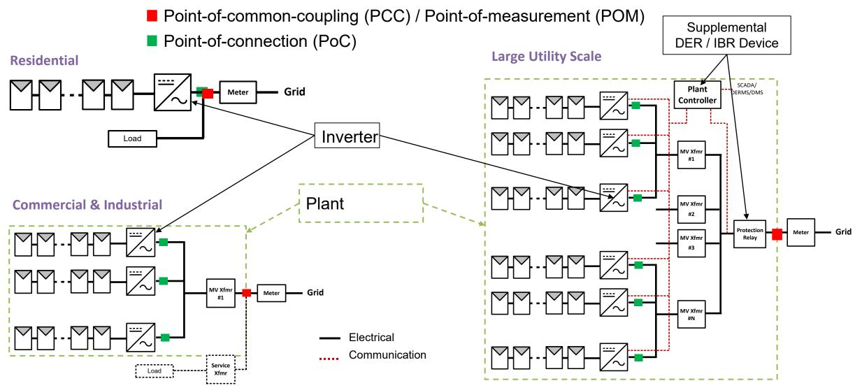
DER Plant-Level Performance Verification and Commissioning Guideline: First Edition. Technical Update. EPRI. Palo Alto, CA: December 2020. 3002019420 Source: EPRI For larger-scale DER and large-scale IBR, plant controller can be critical to meet the IEEE 1547-2018 / 2800 requirements at PCC / POM.
