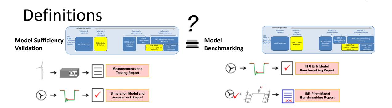
The dynamic process of **comparing measurements**<sup>1</sup> with **simulation results**<sup>2</sup> for the assessment whether a model response adequately mimics the measured response for the same event/disturbance and external power system conditions.
