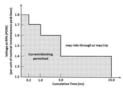
The *IBR unit*'s TOV ride-through capability may differ from the *IBR plant*'s TOV ride-through requirement specified in this subclause. The *IBR plant* design should coordinate an *IBR unit*'s TOV ride-through capability with surge protection implemented within the *IBR plant* to allow the *IBR plant* to meet specified TOV ride-through requirements.
