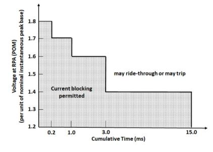
The *IBR unit*'s TOV ride-through capability may differ from the *IBR plant*'s TOV ride-through requirement specified in this subclause. The *IBR plant* design should coordinate an *IBR unit*'s TOV ride-through capability with surge protection implemented within the *IBR plant* to allow the *IBR plant* to meet specified TOV ride-through requirements.
