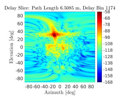
Synthetic apertures can provide high-resolution measurements in dense scattering environments
